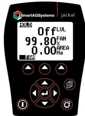
For the machine to operate, the **RUN/HOLD** in the top left of the screen, must display **RUN**.
