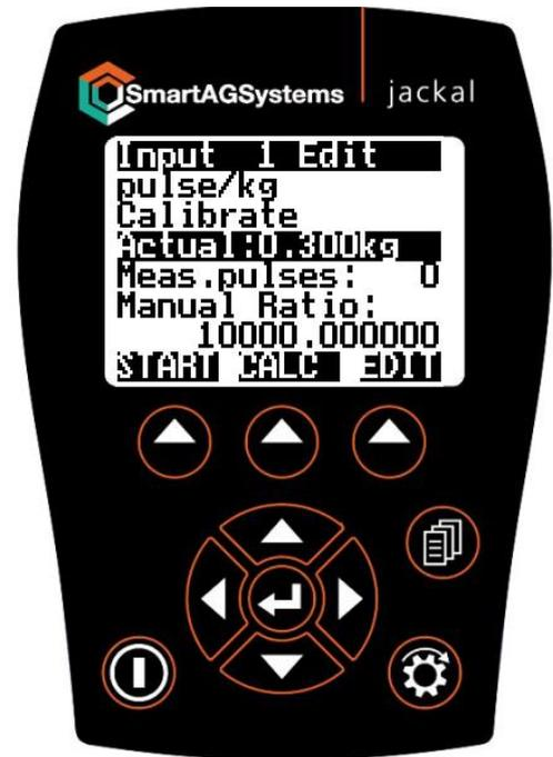
To confirm the actual weight that has been entered, now press **CALC** to work out the new ratio.
