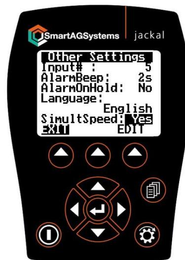
When simulated speed is turned on, this function is now available when scrolling through the screen functions using the PAGE button.
