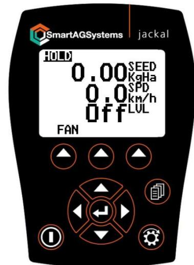
When **FAN** is highlighted, the fan should be running.
