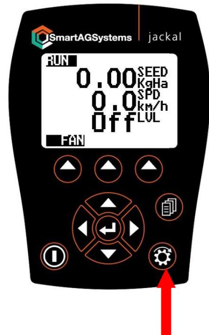
As the machine is about to start work, set the application rate required. This can be done by selecting one of the two pre set "quick rate" buttons.
