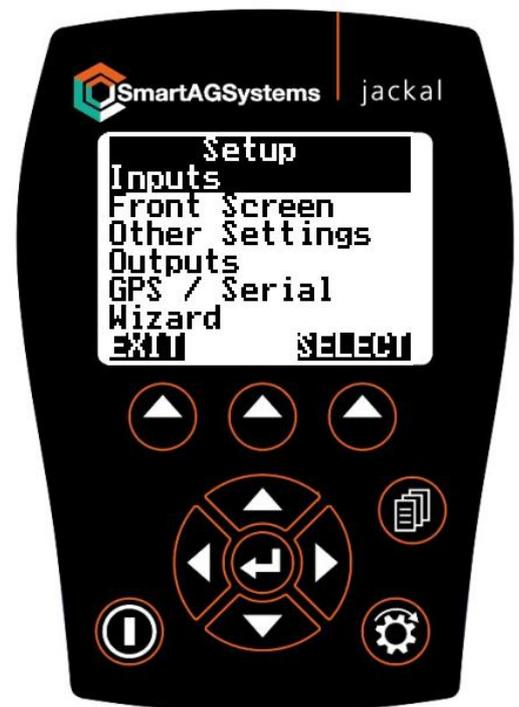
Using the navigation keys, scroll down to the implement width.
