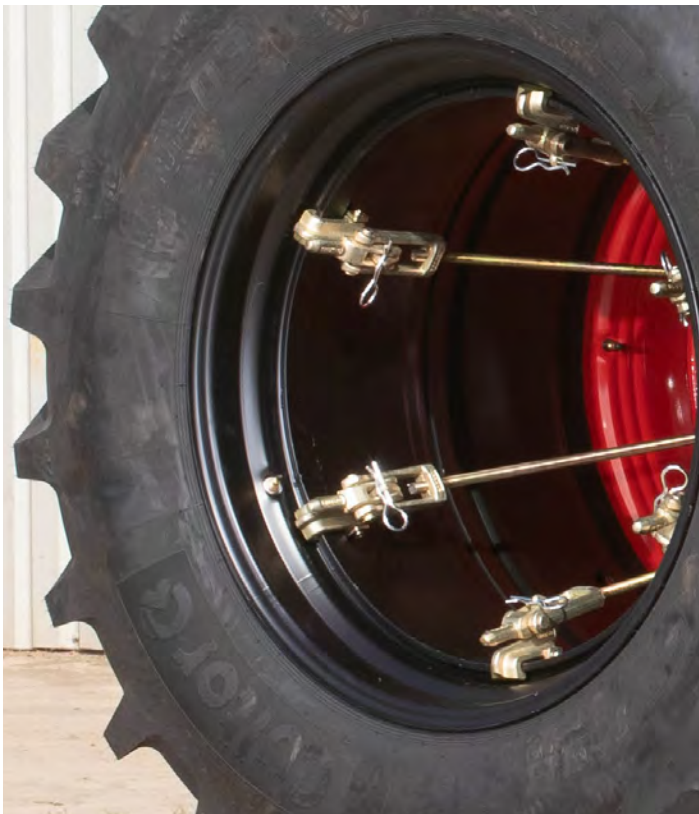
Image of tractor wheel showing spacers fitted
