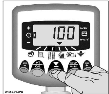
Figure 14 : View Drilling Rate (kg/ha)
