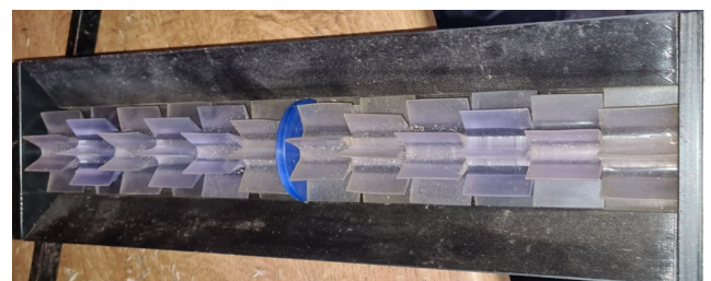
Outlet feed block with 3 grass seed rollers fitted per outlet on a Maxi Jet 4
