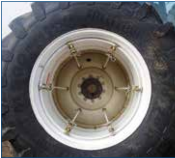
Image of tractor wheel showing spacers fitted
