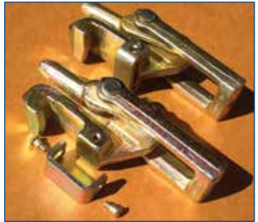
Close up image showing spacer fitted and removed
