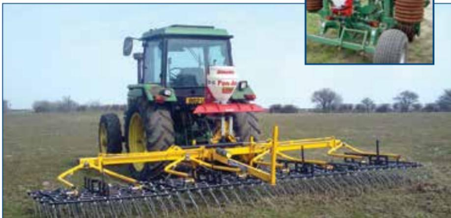
**Grass Seed Deflector.** This easily attached, adjustable, all steel deflector gives a more accurate and controlled placement of grass seed when re-seeding or overseeding pasture with a tined grass harrow. It provides adjustable width and depth of spread, and will deflect seed down into the tines of the harrow – especially useful in windy conditions. It is suitable for use with harrows 3 – 6m wide, and supplied with a grass agitator as standard.
